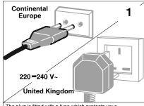
The plug is fitted with a fuse which protects your television. If your television does not work, the fuse may be blown. In this case, replace it with an identical 5 Amp ASTA or Ir BSI (BS 1362) certified fuse.
